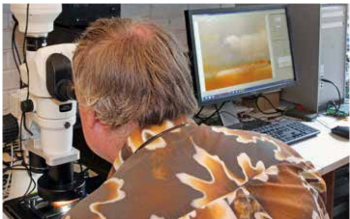
Prof Robert Weston at his studio near Cardiff, south Wales. He is using the Nikon Metrology SMZ1270 stereoscopic microscope fitted with a x200 zoom lens and a Nikon DS-Ri2 camera to view an agate crystal. An image of it can be seen on the screen of the linked PC.
