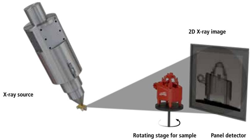
X-ray scans are taken at discrete positions of the rotating stage. Afterwards all slices are reconstructed to a 3D CT volume.
