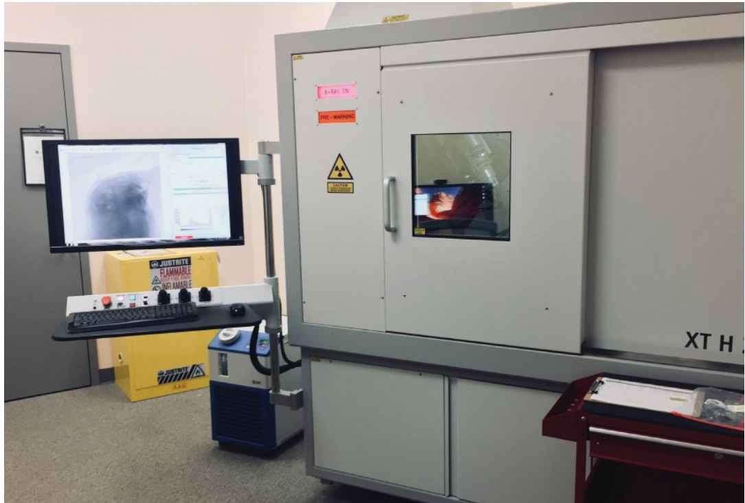
Figura 1. Sistema micro-TC de 225 kV, XT H 225 ST de Nikon Metrology
