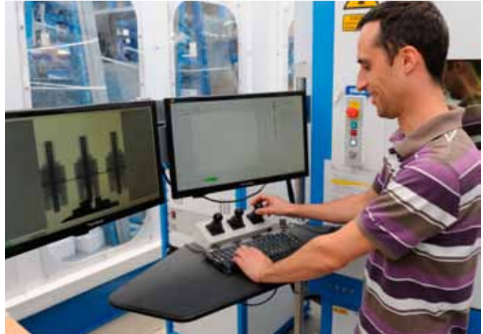
The X-ray images show the interior of the components.
