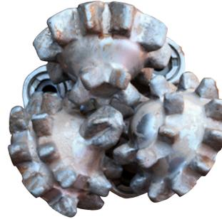
■ A tricone rock drill bit - used for rock abrasion to extract ground water, oil and gas.
