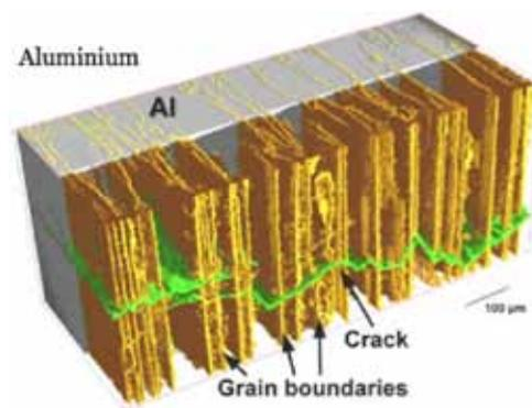
*Fatigue damage in high strength Al-alloys, as used in high pressure gas containment systems.*
