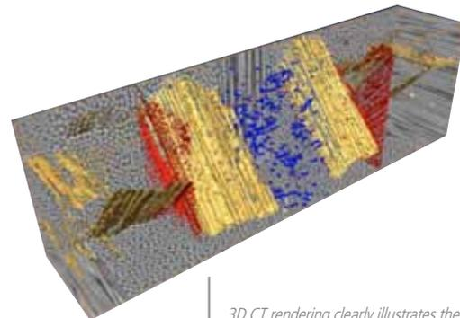
*3D CT rendering clearly illustrates the fibre orientation and damage that are observed in laminates.*
