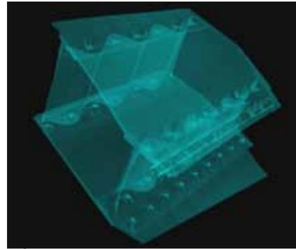
*3D rendering of an aircraft wing part (~400mm across) scanned using a 450kV X-ray source and a curved linear detector array.*
