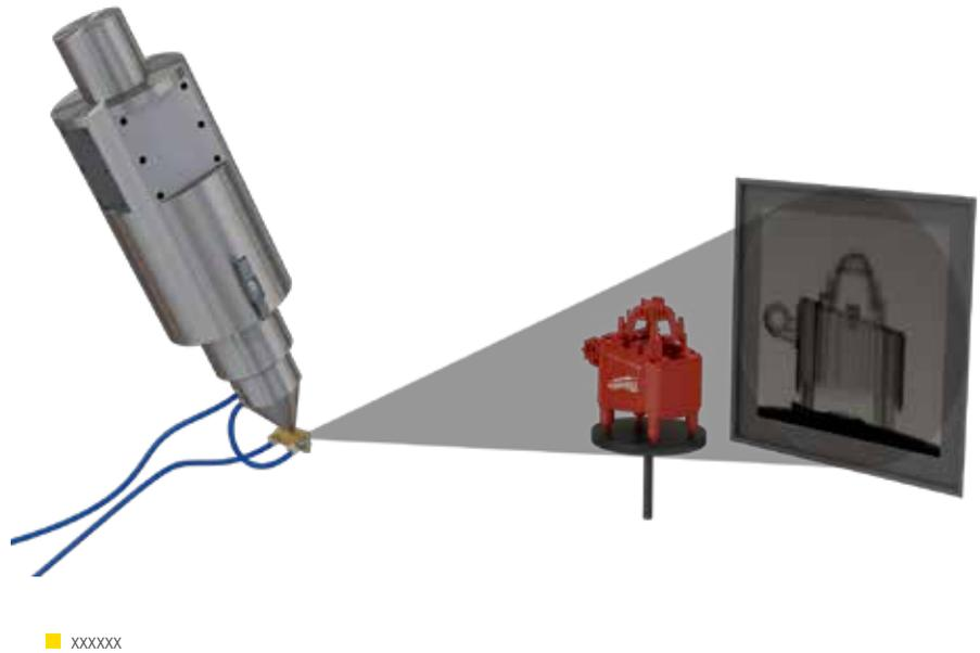
largest offering, a combined 225/450kV microfocus X-ray and computed tomography system. The system's powerful source, walk-in bay, and panel shift capability allow Chesapeake Testing the versatility to inspect larger components that typical cabinet CT systems are unable to accommodate. This large-scale system gives Chesapeake Testing the capability to image large objects up to 37 inches in diameter.
