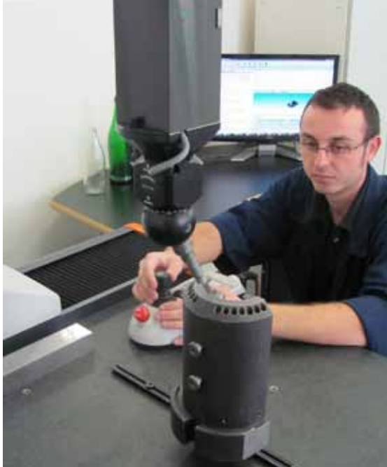
Final inspection throughput of a glass bottle mould is tripled by using CNC multi-sensor CMM.
