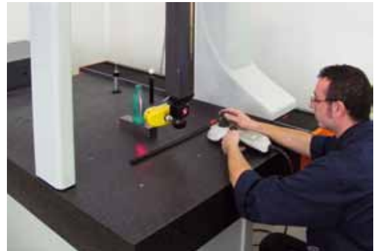
The LC50Cx digital line scanner on the CMM inspecting a resin model of a Coca-Cola bottle.
