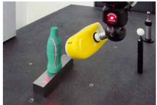
LC50Cx digitizes nearly all surfaces including reflective material
