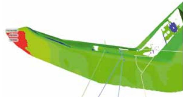
*Wall thickness, clearance, 3D angle and flatness analyses are performed using PolyWorks IMInspect*
