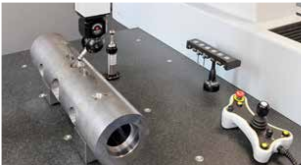
One of the EN8 gas flow meter cylinders, measuring 130 mm in diameter by 550 mm long, being inspected in a 9-minute cycle.
