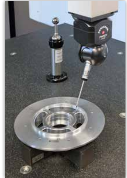
The aluminium turbine component being inspected in a cycle time of 10 minutes at Nisan Engineering, Leicester.
