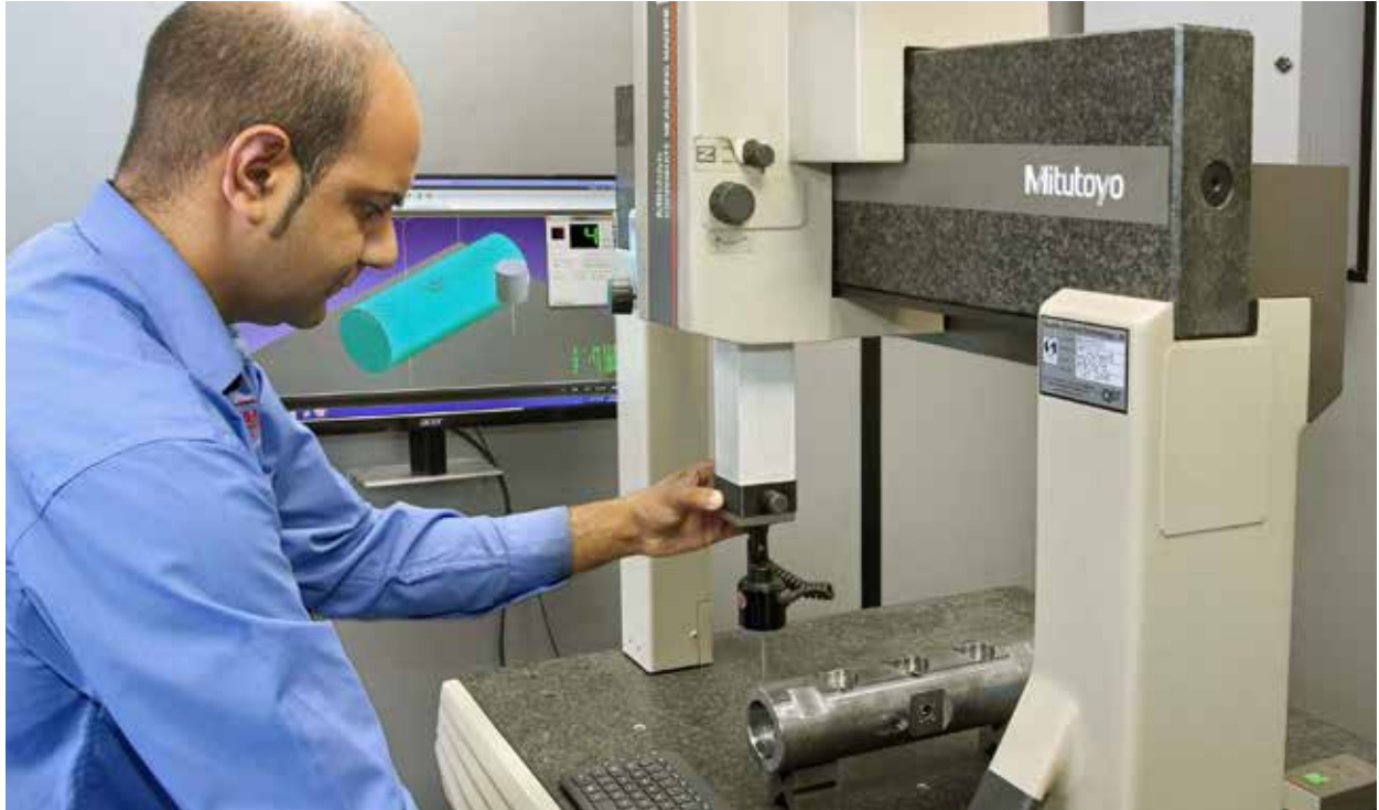
The same cylinder being inspected on the manual Mitutoyo CMM, retrofitted with CMM-Manager software.
