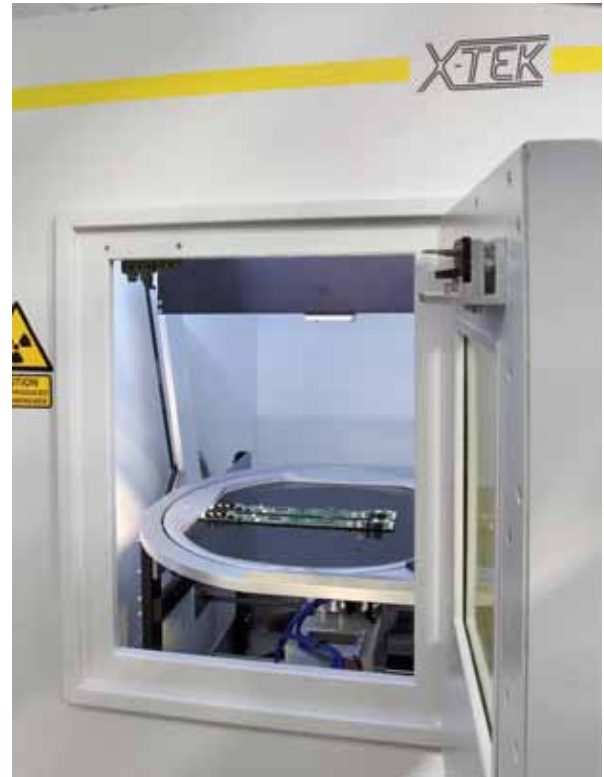
PCBA assemblies positioned above the X-ray source, ready for inspection
