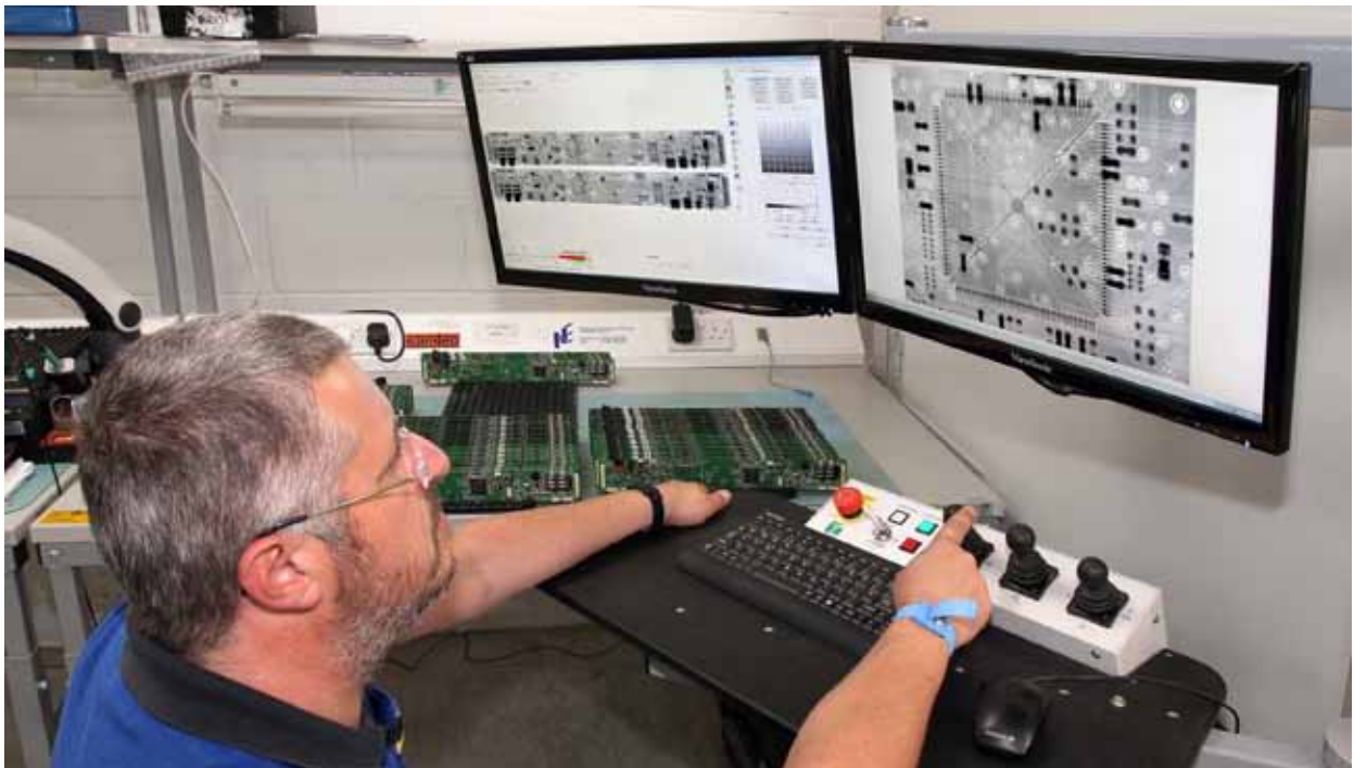
Dave Roe checking the X-ray results. The dual display facilitates combined measurement and real-time analysis.
