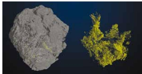
*Micro-CT scanning helped lay bare the rock's beautifully shaped gold fronds and calculate their volumetric fraction.*
