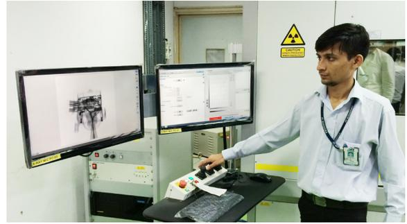
■ The screen shows live images of a lever combination switch and its internal features.
