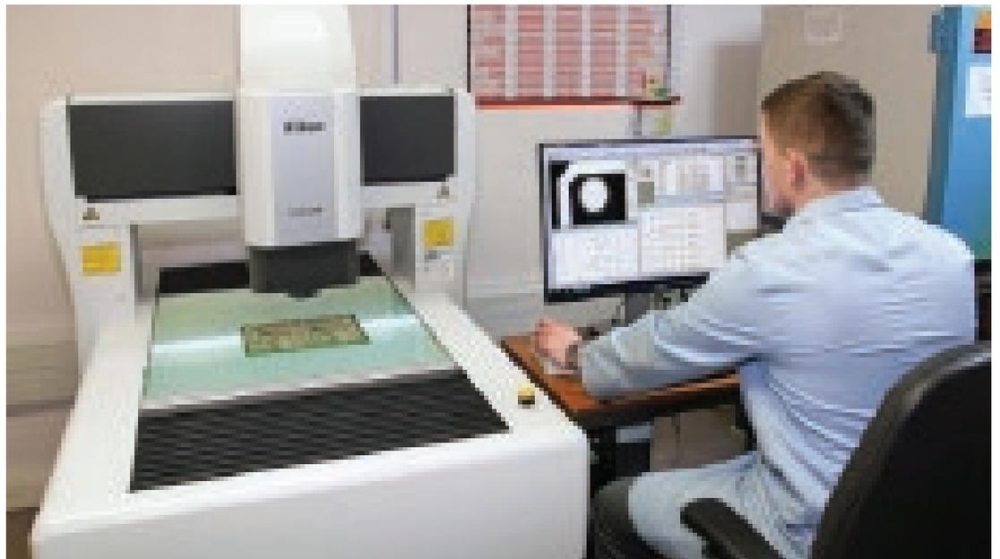
In use at the University of Hartford for training graduates and local engineers, the Nikon Metrology iNEXIV VMA-4540 CNC video measuring system with Renishaw TP20 touch-trigger probe has a large field of view, long working distance and wide XYZ strokes, enabling automatic measuring of a wide range of 3D components.
