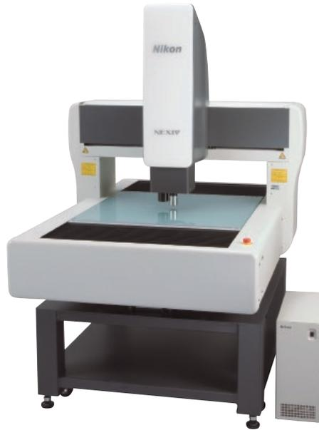
Another Nikon Metrology CNC video measuring machine with 15x zoom optics in use in the metrology laboratory at Uhart is the VMZ-R4540 Type 1. Its magnification, AF and LED episcopic / diascope illumination can be finely adjusted, while working distance and field of view are both large.
