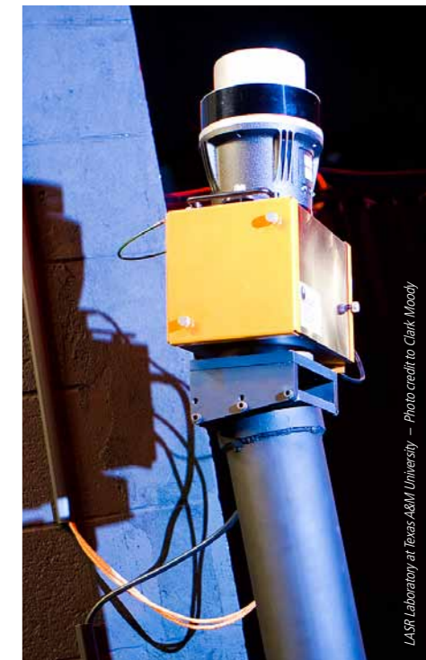
Six fixed iGPS transmitters cover the 2000 square foot experimentation area.
