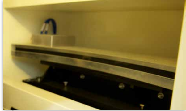
The curved linear diode array detector (CLDA) optimizes the collection of X-rays by eliminating scatter phenomena that typically corrupt 2D radiographs of blades and other metal parts.
