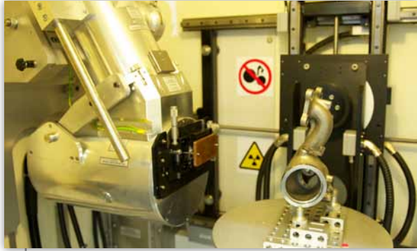
The XT H 450 X-ray source is suited to scanning small castings to gain an insight into the inner details of the part.
