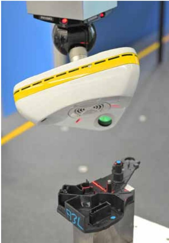
*The digital Cross Scanner features 3 laser lines from different angles to measure complex shapes with a minimal number of PH10 head rotations*
