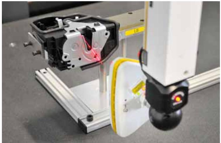
*The Cross Scanner digitizes complex multi-material assemblies in an easy and fast inspection process.*
