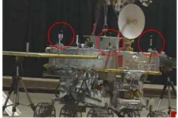
Nikon's iGPS equipment (iGPS sensors are encircled) are used during laboratory tests for e.g. trajectory verification
