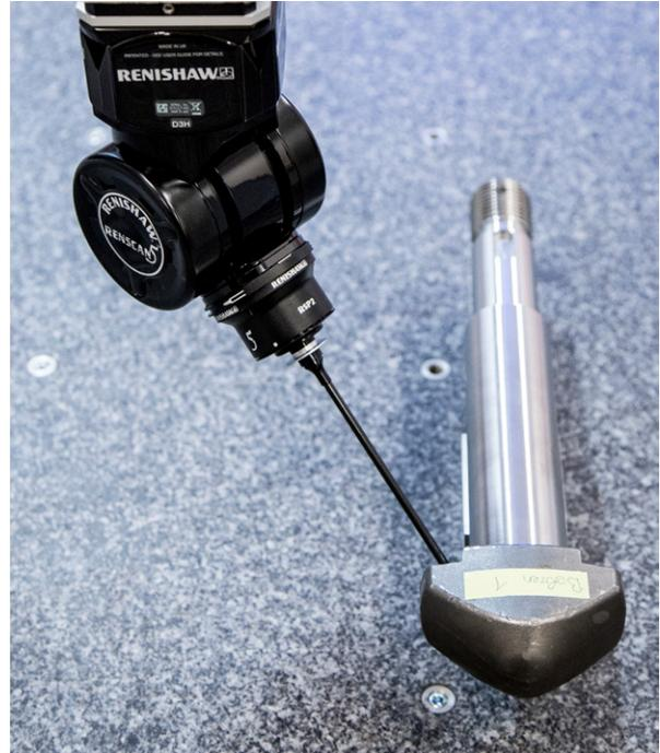
■ The REVO probe enables 3D contact scanning at very high speeds without any problems.
