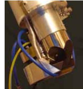
A microfocus X-ray source equipped with a rotating target increases X-ray flux by a large factor, allowing for faster data acquisition or higher data accuracy
