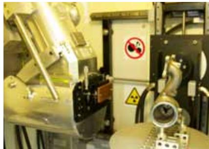
*The XT H 450 X-ray source is powerful enough to scan small castings with micron accuracy*
