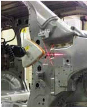
*The Nikon Metrology XC65D laser scanner captures geometric features from 3 sides simultaneously.*
