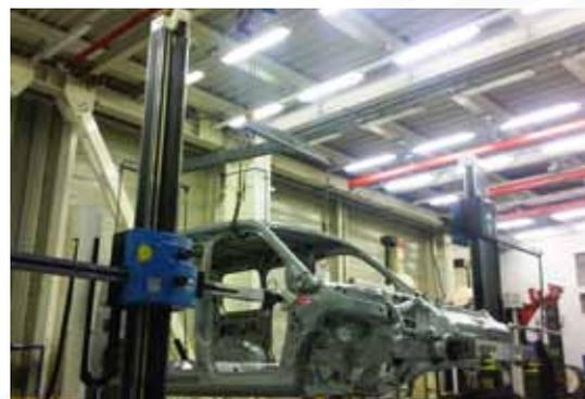
*Ford Otosan successfully made the shift to the XC65D laser scanner for mainstream vehicle body inspection.*
