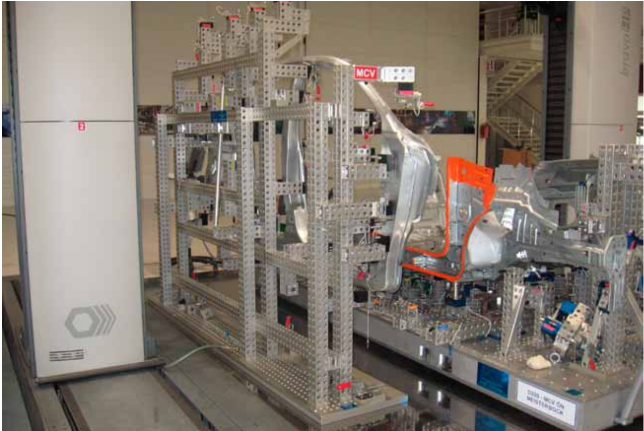
The meisterbock is a complex fixture to verify the assembly of different panels of a prototype vehicle
