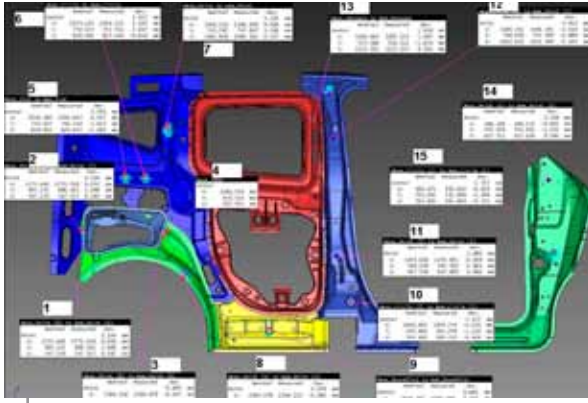
Laser scanning of car body panels yields a wealth of data, enabling virtual assembly of body-in-white and geometry evaluation in software.
