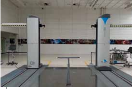
Nikon Metrology XC65Dx-LS Cross Scanners are fitted to a Hexagon double-arm CMM at the Bursa factory of TOFAŞ.
