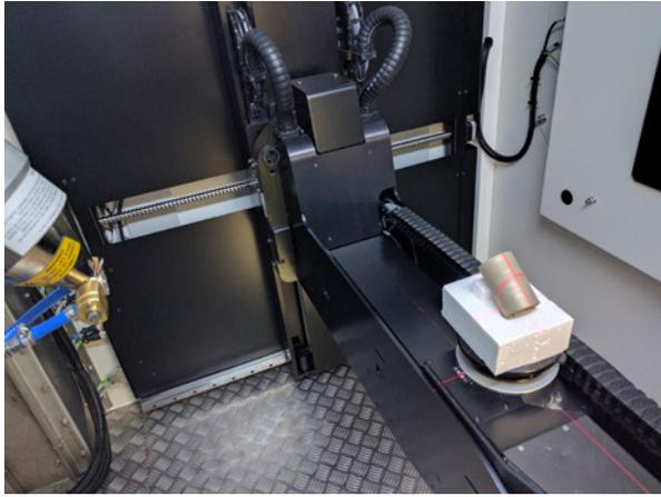
■ A part is placed on a rotate stage and 2D X-ray images are taken at incremental angles. Then the 2D X-rays images are reconstructed into a 3D model.
