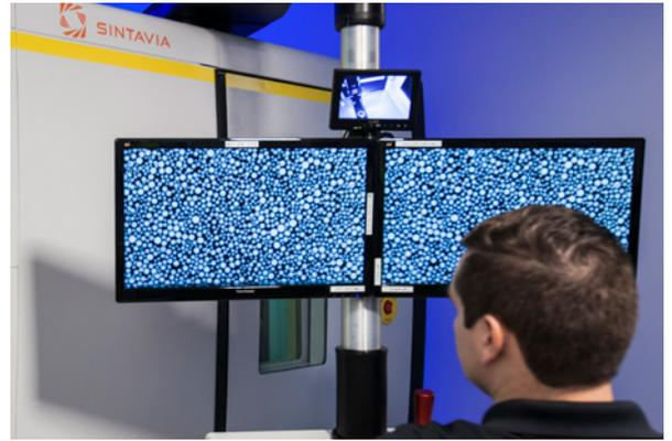
■ The micro-focus CT system allows to visualize individual metal powder particles.
