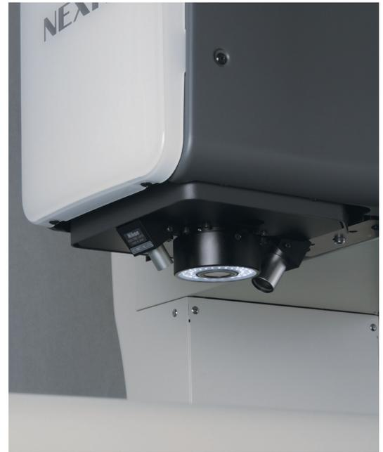
lens that has a working distance that is suitable for all of the measured features. You'll need a lens with a working distance that can get close enough to deeper features, without colliding with higher features.
