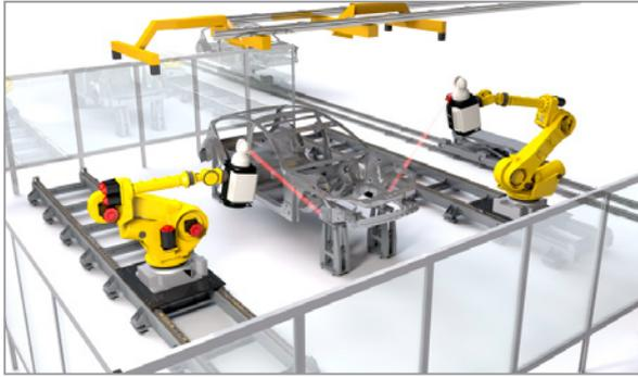
■ Line-side inspection: A car body is taken from the line and fully inspected. Two or four robots guarantee the highest inspection productivity. After inspection the body is re-inserted into the production line.
