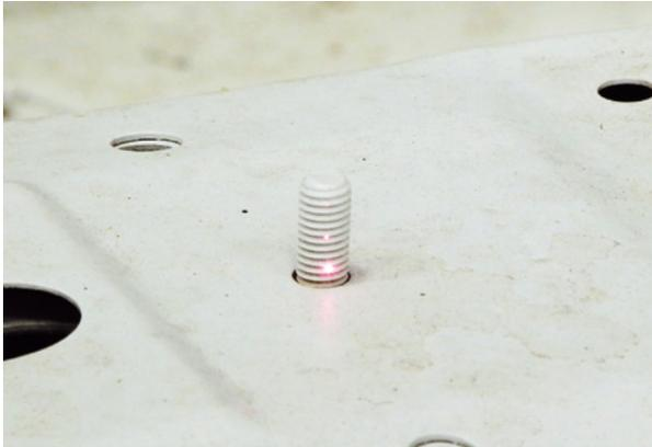
■ Features such as holes, slots, pins, studs can be quickly inspected using the Laser Radar
