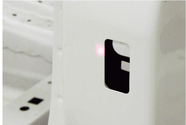
component, sub-assembly and full body checks in the CMM room. Multiple turntables can be tended from a single Laser Radar reducing measurement dead-time while loading or changing fixtures. This approach optimizes productivity and reduces the traditional CMM room bottleneck.
