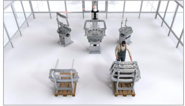
■ Component inspection: a single Laser Radar on a lift inspects front and back of multiple components on rotate tables.
