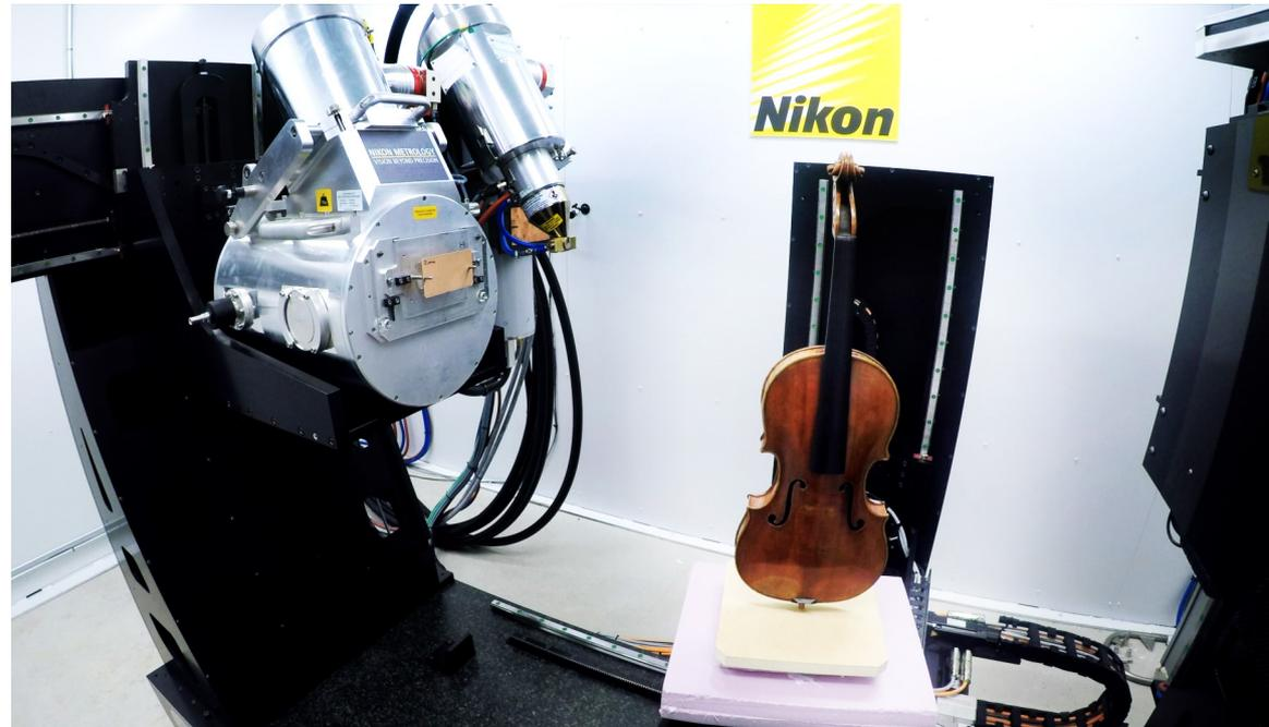
An 18<sup>th</sup>-Century Venetian violin being scanned by Nikon Metrology's large envelope M2 micro focus X-ray/CT inspection system.
