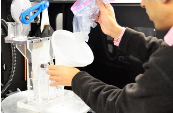
■ Parmesh loads an in-situ shaking mechanism inside the CT system with glass beads for a 4D CT experiment simulating the Brazil Nut effect.
