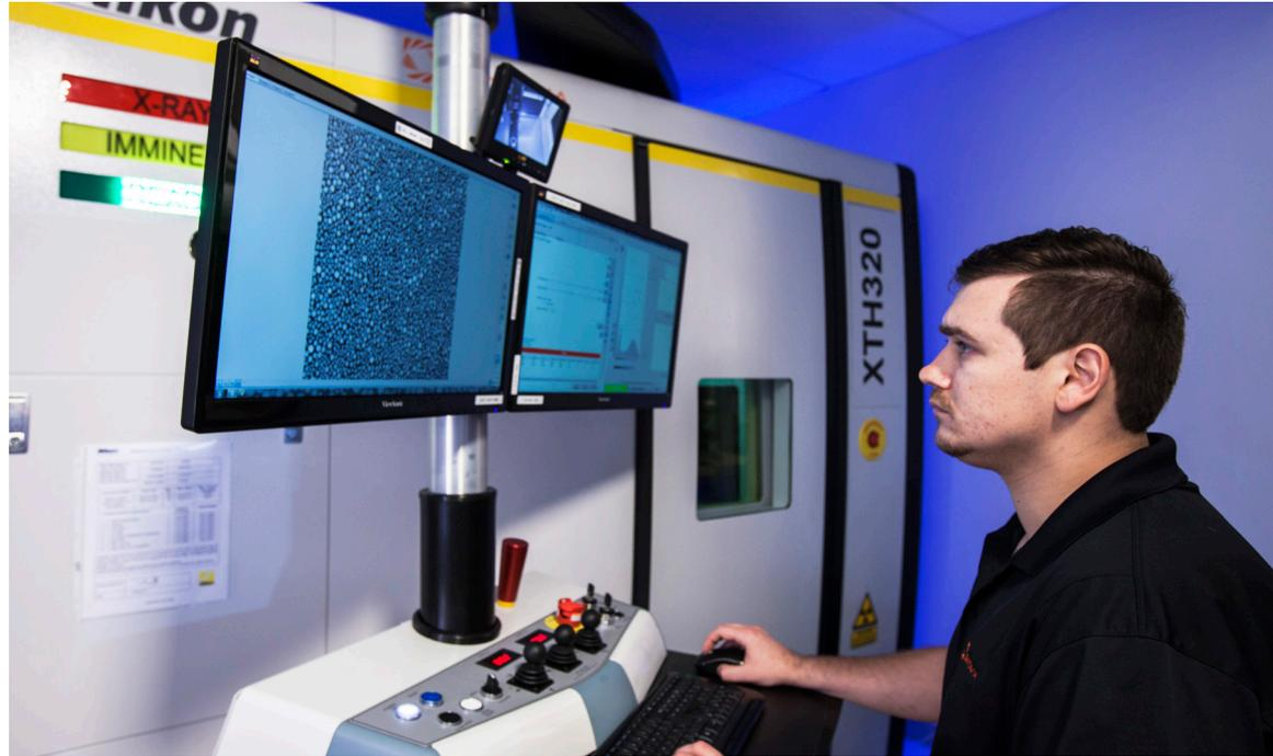
Metal powder for additive manufacturing being inspected using Nikon Metrology micro CT scanner at Sintavia
