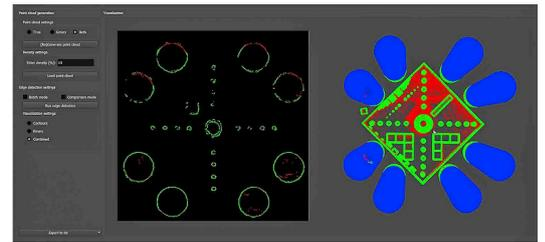
At RISE, STL files are compared to images from the 3D printer in real time or after printing. 2D and 3D visualisation of the build process and its defects allows operators to explore the component and quickly find deviations.
