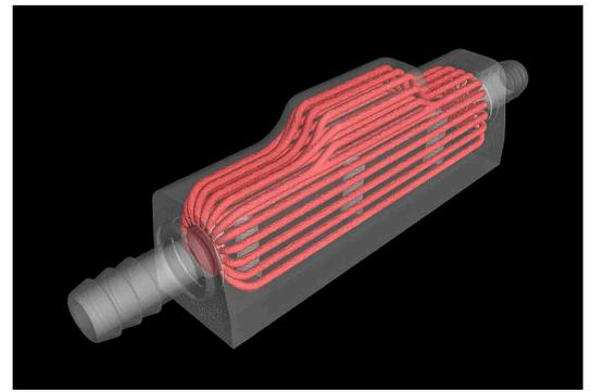
The component was scanned in 50 minutes to reveal its internal structure. Voxel size is 100 µm / 39 µm with PE 1611 helical scanning.
