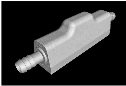
An tool steel component measuring 115 x 45 x 35 mm additively manufactured at RISE.
