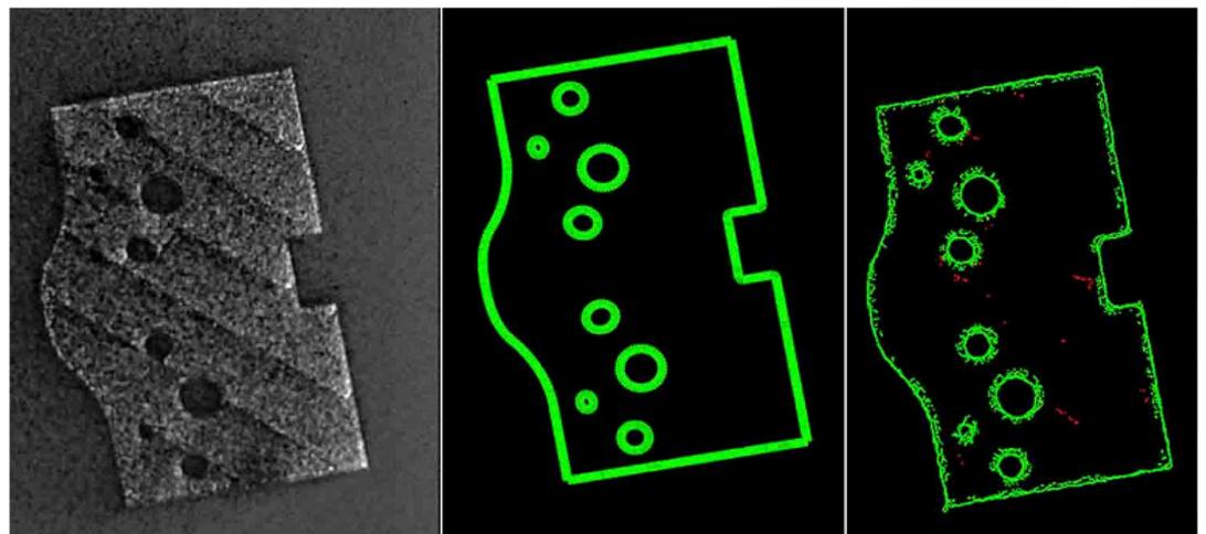
Using RISE software, an original image (left) is compared to its CAD model (centre), resulting in a deviation detection image (right) where pixels in red show potential deviations.
