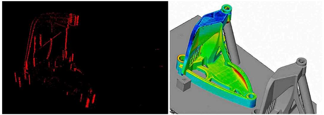
Left: results from the deviation detection software using high resolution images from the 3D printer. Right: the CT scan performed after printing shows similar deviation around the overhang and outside edges.
