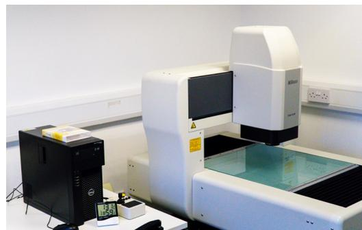
probe to the iNEXIV. It enables measurement of features on more complex 3D parts, where probing can complement the video measurement making the system even more versatile. Both optical and tactile measurements can be combined in a single inspection cycle, providing the speed and accuracy of video measurement system with the additional benefits of a CMM.
