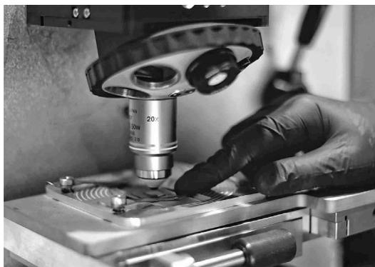
Nikon optics and illumination components used to industrialise NETA's ASOPS photo-acoustic imaging system, JAX, for measuring thin films to nanometer accuracy.
