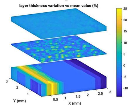
Typical results derived from a thin film using the JAX characterisation system.
