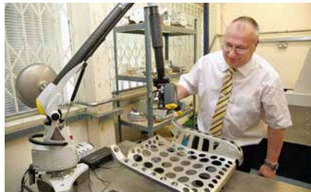
*The MCAx measuring arm with a hand-held laser scanner inspecting part of an aircraft seat.*
