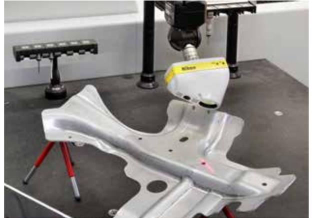
*Close-ups of the Jaguar prototype pressing being inspected using the Nikon Metrology LC15Dx laser scanner head.*
