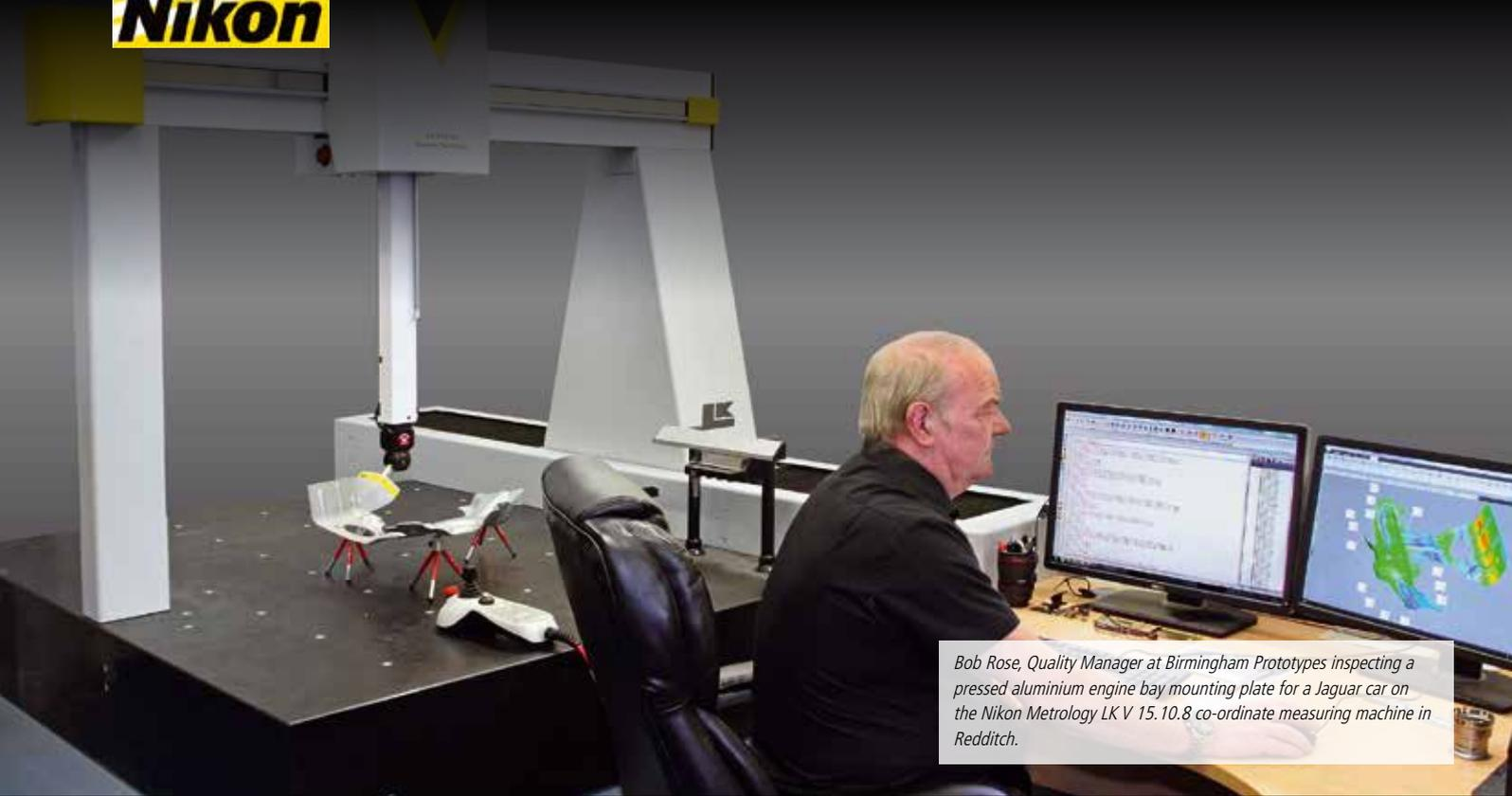
*Bob Rose, Quality Manager at Birmingham Prototypes inspecting a pressed aluminium engine bay mounting plate for a Jaguar car on the Nikon Metrology LK V 15.10.8 co-ordinate measuring machine in Redditch.*
