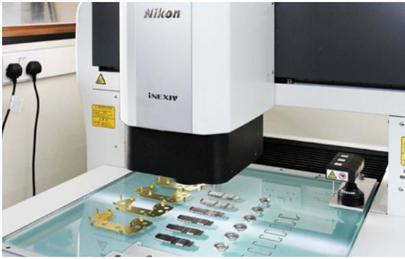
■ Steve Bettridge, quality manager of Berck Ltd, with the Nikon Metrology iNEXIV VMA-4540 multi-sensor CNC inspection machine, which includes video measuring and tactile probing capabilities.
