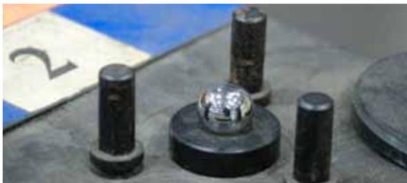
*Detail of tooling ball on rotating table*
