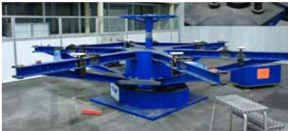
*The huge rotating table is equipped with small tooling balls the Laser Radar measures to reference the table.*
