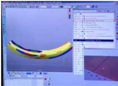
*The color-coded areas graphically illustrate the geometric deviation of the leading edge surface.*
