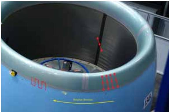
*Laser Radar executes automatic freeform surface and gap & step measurements at every increment of the rotating nose cowl.*
