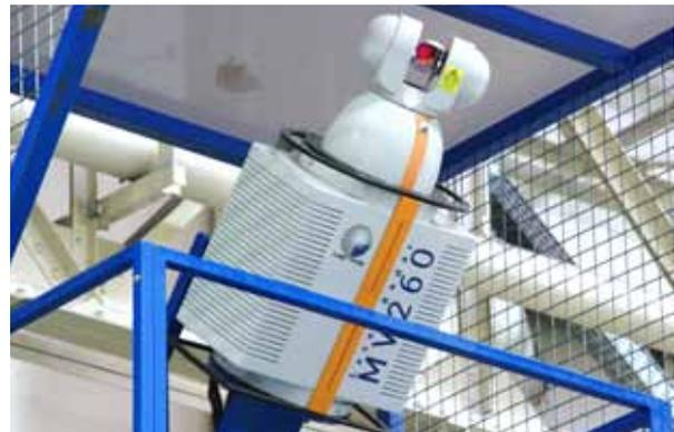
*Airbus opted for an automated Laser Radar inspection cell that drastically speeds up nose cowl inspection.*
