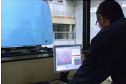
*The Metrolog software synchronizes the rotation of the Airbus nose cowl with the Laser Radar measurements.*
