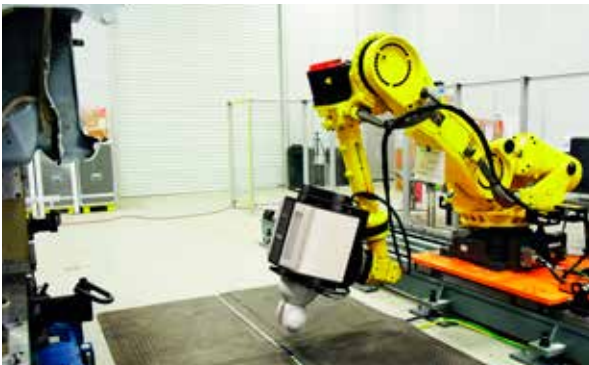
■ In each robot position, the Laser Radar can inspect dozens of features
